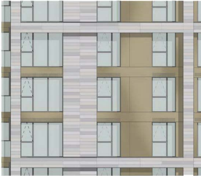
① DETAIL 01 - RESIDENTIAL WEST ELEVATION TYPICAL MODULE 1 : 50
